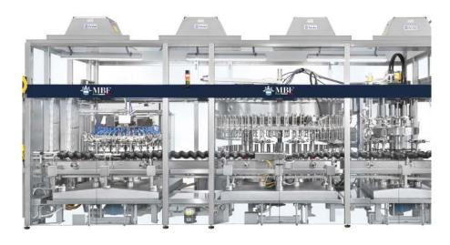
New 12,000bph MBF Filler installed into WW Marlborough Line 4, replacing current Alfatech filler.
