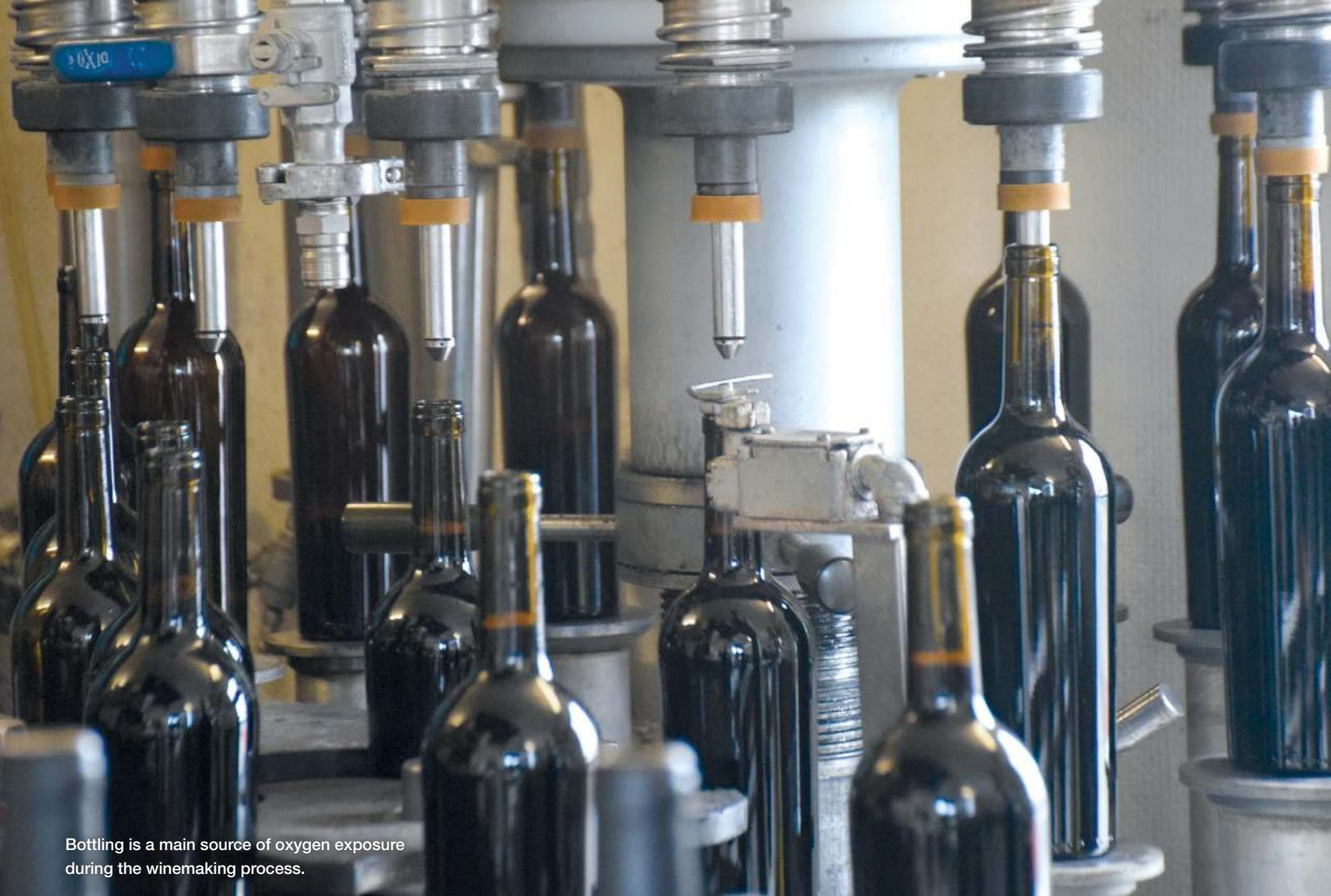
Bottling is a main source of oxygen exposure during the winemaking process.
